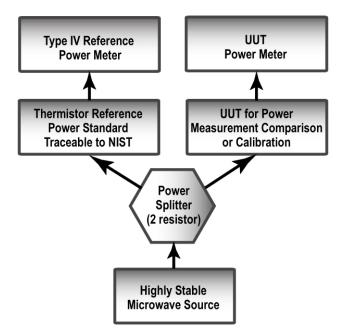
Figure 1 – Block diagram of a Direct Comparison System.
