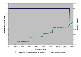
Figure 3 - Graph of signal generator specified output versus typical RF losses for 26.5 GHz System II.
